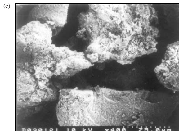
Figure 6. SEM fractographs of (a) HC-HPMA0 graft copolymer, (b) HC-HPMA7 graft copolymer, and (c) HC-HPMA34.
